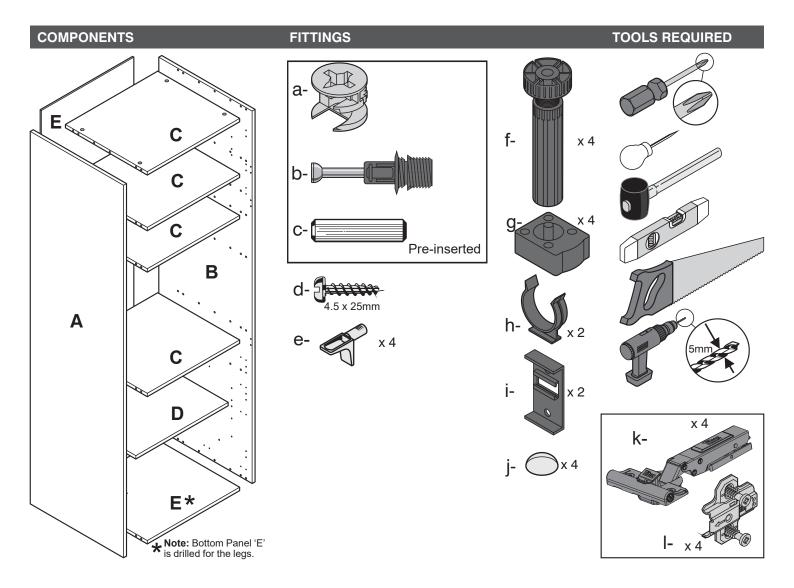
**Important:** The panels must be fitted with the cams positioned as shown.
